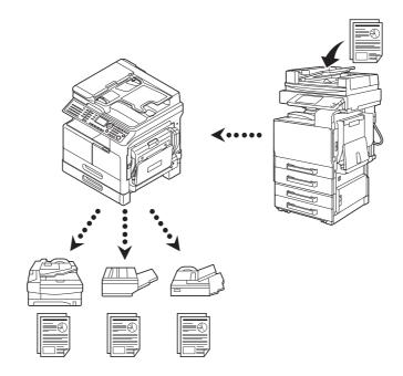
To specify the relay broadcasting, you must register a 4-digit Relay User Box ID and receiving stations (last destinations) in advance. Up to 10 Relay User Boxes can be specified. For details, refer to page 7-19.
