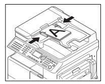
→ A custom-size original can be scanned up to the sizes shown below. Width: 8-1/2 inch (210 mm)<sup>\*</sup> to 11-11/16 inch (297 mm)
