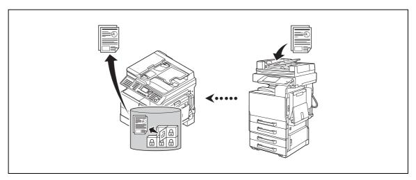
Sending an original to a Confidential User Box of the recipient machine is referred to as confidential transmission, and receiving an original in a Confidential User Box of your machine is referred to as confidential reception.
